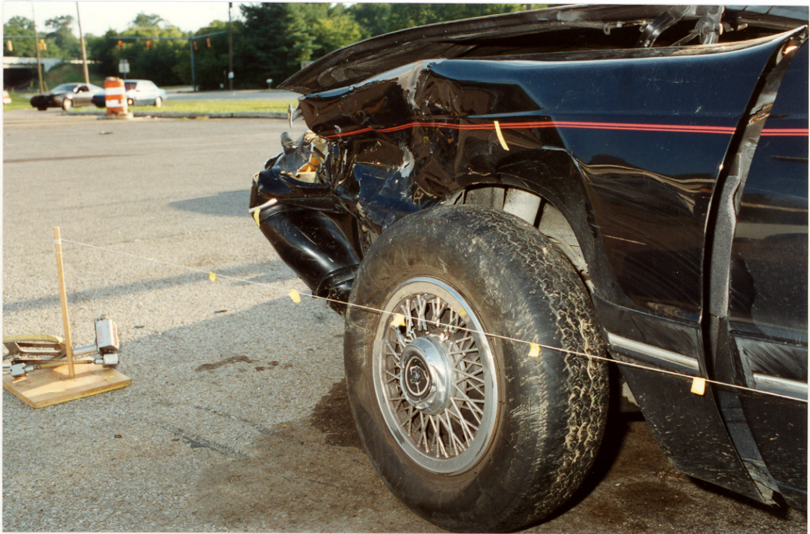
111. View of the primary contact deformation.
